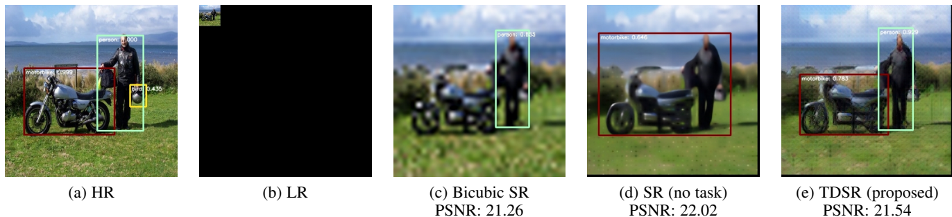
Fig. 1. Scale sensitivity in object detection and the effectiveness of our proposed method (i.e., end-to-end learning in accordance with the mutual improvement of SR and object detection tasks). Images shown in the top row show (a) an original high resolution image, (b) its low-resolution image (here 1/8-size, padded with black), (c) SR image obtained by bicubic interpolation, (d) SR image obtained by the SR model optimized with no regard to detection, and (e) SR image obtained by our proposed task-driven SR method, using the same model as in (d). For each of the reconstructed HR images, we also report PSNR w.r.t. the original. Despite ostensibly lower PSNR, the TDSR result recovers the correct detection results with high scores, in this case even suppressing a false detection present in the original HR input.
